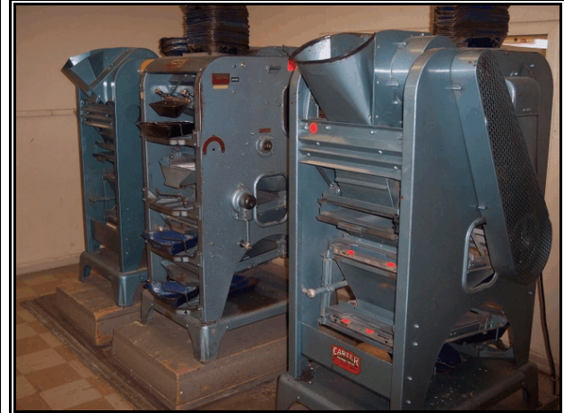
Dockage machines at State Grain Lab separate wheat from chaff
